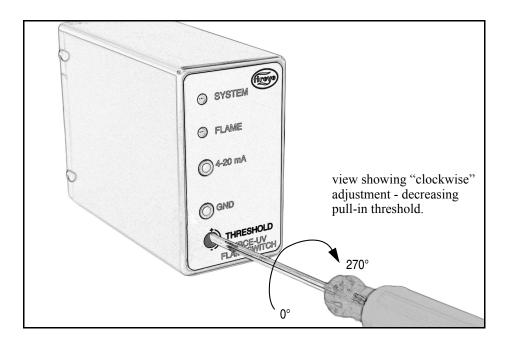
• Apply proper grounding technique when adjusting the threshold potentiometer
