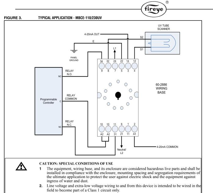
**3.** A 1 amp external fuse is suggested on terminal 10 (flame relay common) for over-current protection
