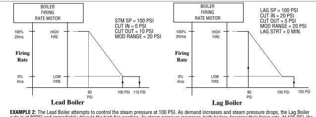
Lag Boiler cuts in at 80PSI and immediately drive to the high fire position. As steam pressure increases, both boilers decrease their firing rate. At 105 PSI, the Lag Boiler cuts out. It won't cut in until steam pressure again drops to 80 PSI. The Lead Boiler cuts out at 110 PSI and cuts in at its steam pressure set point (100 PSI).
