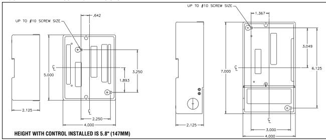
FIGURE 2. MOUNTING DIMENSIONS
