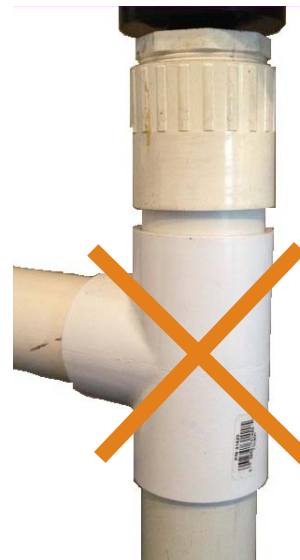
Avoid the use of a tee within the stand pipe. A tee can create false signals that will negatively effect the sensor's performance.
