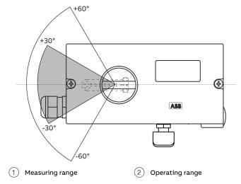
Figure 9: Measuring and operating ranges of the positioner
