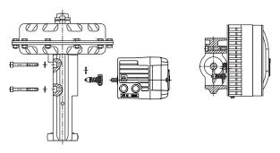
Figure 4: Integral mounting on control valves
