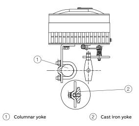
Figure 2: Mounting to linear actuators in accordance with DIN / IEC 534
