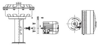
Figure 5: Integral mounting on control valves with adapter plate
