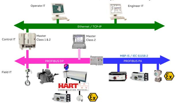
Figure 8: Communication via PROFIBUS®
