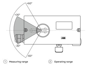
Figure 9: Measuring and operating ranges of the positioner
