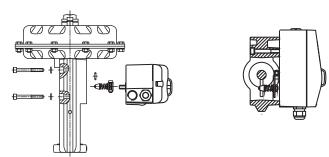
Figure 4: Integral mounting on control valves
