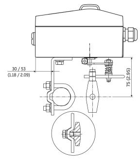
Figure 14: Mounting to linear actuators in accordance with DIN / IEC 534
