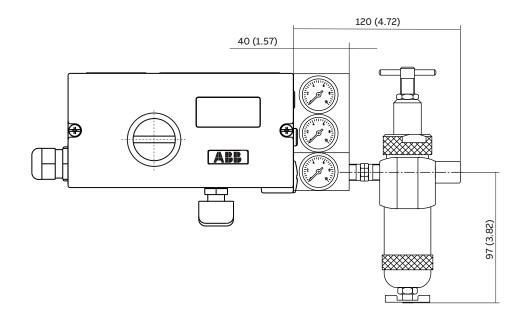
Figure 16: Positioner TZIDC-110 with mounted pressure gauge block and filter regulator
