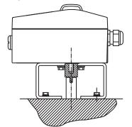
Figure 3: Mounting on rotary actuators in accordance with VDI / VDE 3845
