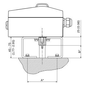
\* Dimensions A and B depend on the rotary actuator
