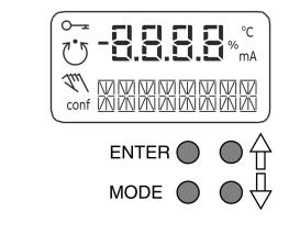
Figure 7: LCD display with operating buttons
