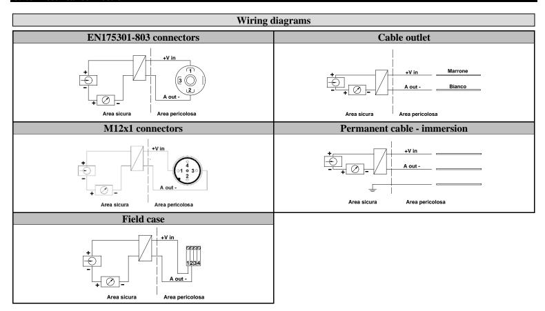
The transmitter's metal case must always be connected to the earth using the threaded connector for the process, in order to protect it against fluctuations due to electromagnetic fields and electrostatic charges. If this cannot be done, connect the transmitter to earth using the connector and the shield on the cable.
