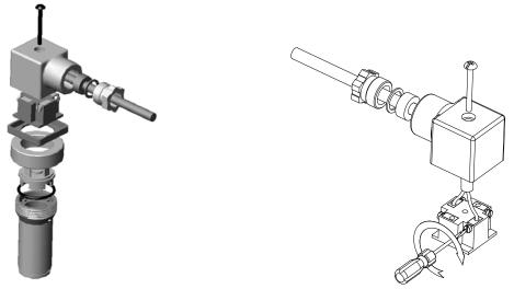
Figure 1 - Exploded view of the connector
