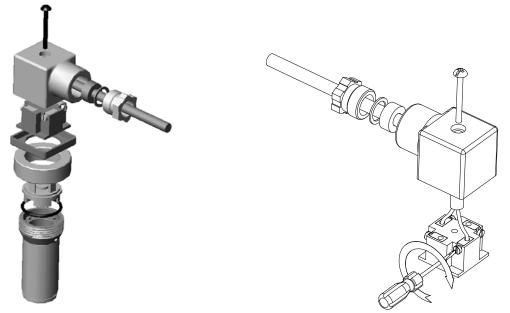
**Figure 1** – *Exploded view of the connector*
