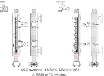
Figure 3.6-1 KM26 with Level Switches
