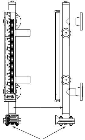
Possible grounding locations with a pipe clamp, pipe strap or ring terminal on flange stud
