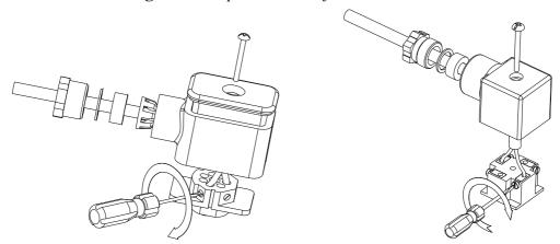
**Figure 2** – *Wires connections*
