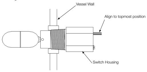
Figure 2 – Installation of MS10 Electrical Contacts
