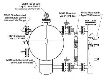
Sample Application Using ABB Inc, K-TEK Level Switches
