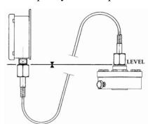
tractions. Do not carry the measuring system at the capillary. Capillary kinking and/or fracture can cause an inner bore throttling increasing the response time or they can cause the instrument failure totally compromising the instrument operation. Capillary
