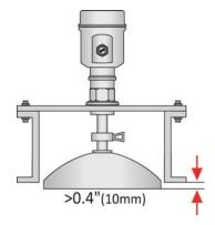
The sensor can be installed within the riser as long as the media has a strong reflective property (dielectric constant) providing a strong echo return. The below information describes the maximum distance that the antenna can be recessed within a riser based on the diameter and height of the fitting.
