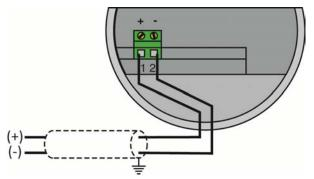
The sensor should be wired with shielded 2-conductor cable (16 to 22 AWG) to protect from electromagnetic interference. If using a liquid tight connector, select a cable with an outer diameter that is designed to ensure an effective seal with the connector [typically between 0.20" to 0.35" (5 to 9 mm)].
