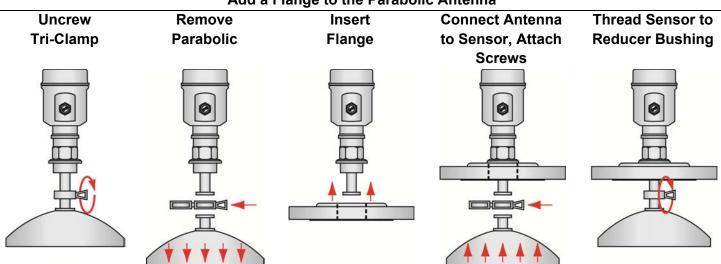
Add a Flange to the Parabolic Antenna
