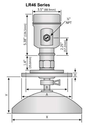
LR46 Flange Parabolic Series Antenna Dimensions
