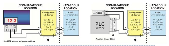
Note: Always refer to the Control Drawing 301901 for further wiring
