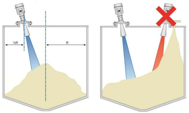
Avoid installing the sensor above the filling stream to avoid interference to the radar pulse. Locate the sensor away from the filling stream.
