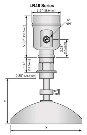
LR46 Threaded Parabolic Series Antenna Dimensions
