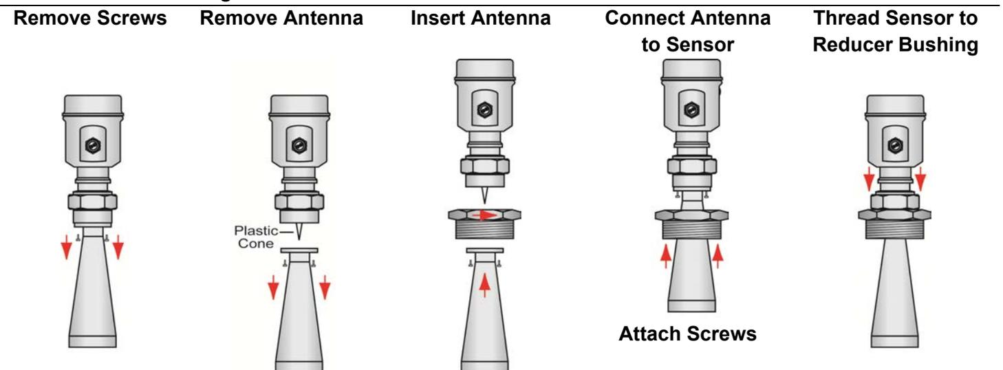
**LR46 PARABOLIC ANTENNA PREPARATION**
