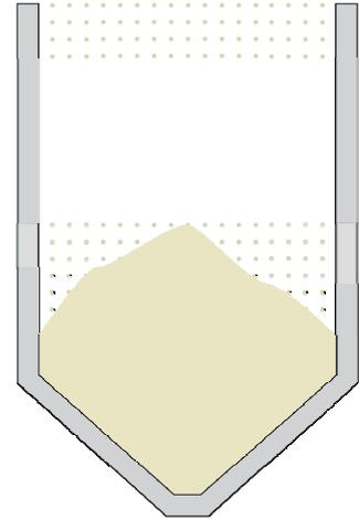
**Significant Powder / Dust** – occurs when the air space is filled from the media to the top.
