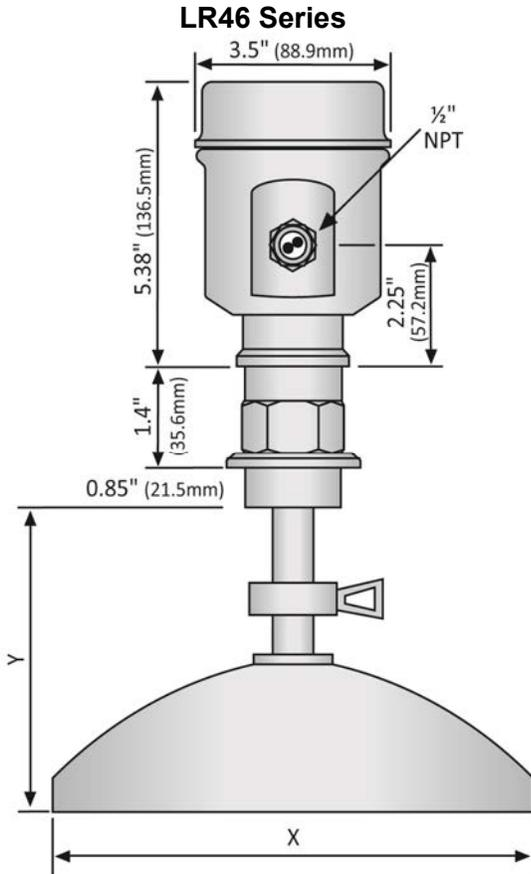
**LR46 Threaded Parabolic Series Antenna Dimensions**
