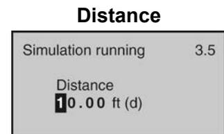
This method uses distance from the sensor's measurement location to set the current output (4-20mA) between the Empty and Full Configuration values.
