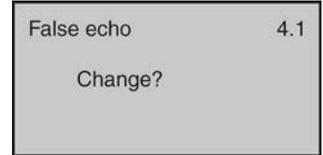
and stores those identified as false into the False Echo Curve, so they will not be considered in the level measurement. **Note:** A False Echo Curve should only be performed when the tank is empty so that all false reflections will be detected.
