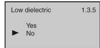
The **Low Dielectric Medium** function has the following settings (*and should not be performed without first consulting with the factory*):
