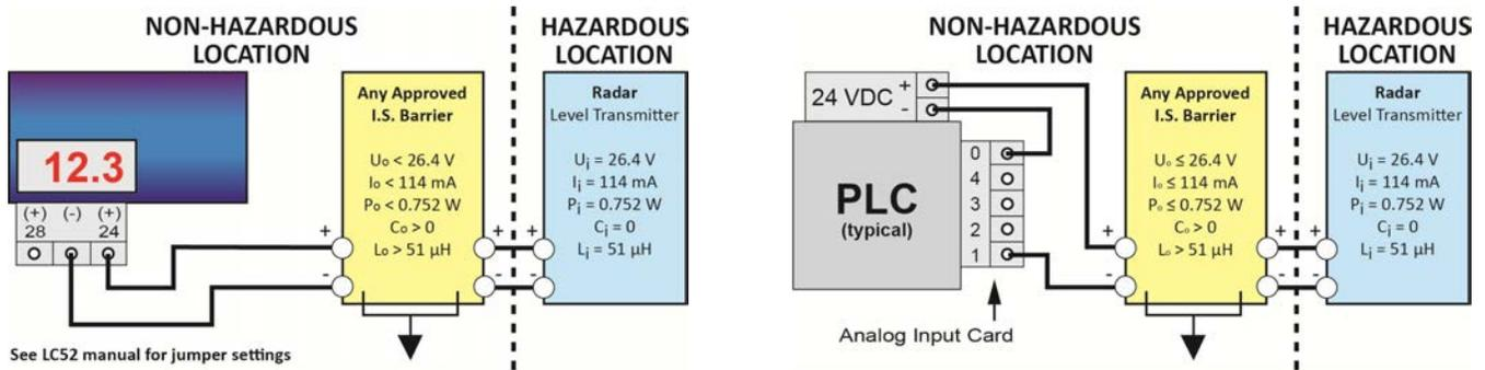
**Note:** Always refer to the Control Drawing 301901 for further wiring
