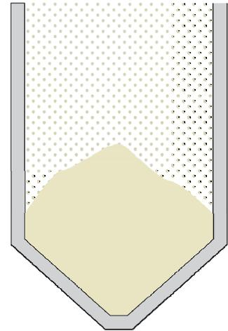
**SOLIDS WITH LARGE ANGLE OF REPOSE**
