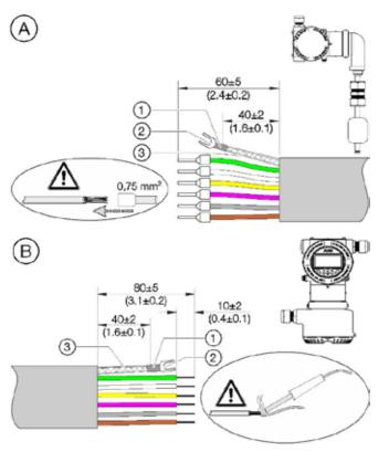
Figure 2 Signal cable dimensions in mm (inch)
