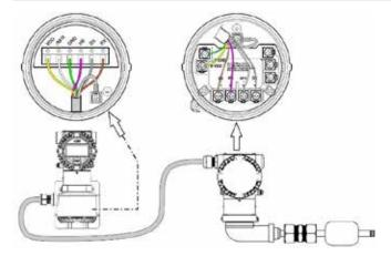
Figure 3 Remote version: connecting the signal cable
