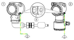
Figure 4 Ground connection on transmitter housing
