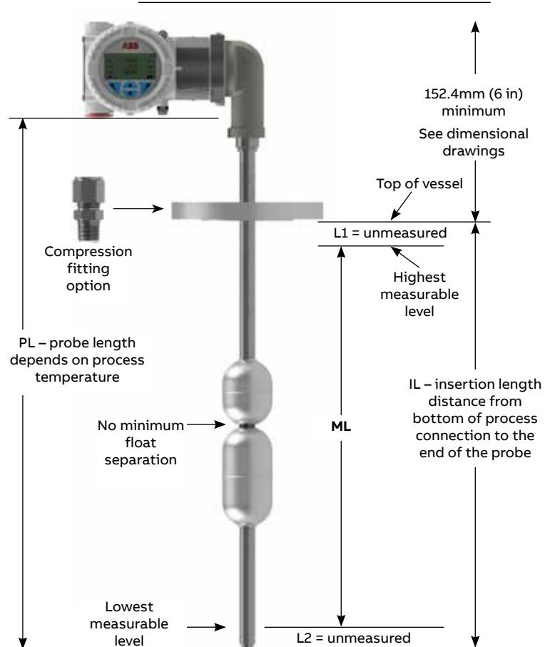
\* Magnet placement and float length determine final dimensions.
