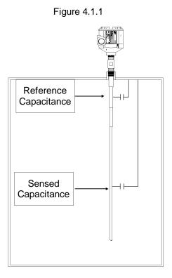
During normal operation, several factors will be taken into account which will affect the action of the relays within the KCAP300. (For this explanation, we will have the Fail Safe set to Low.) When the KCAP300 is calibrated the software establishes a baseline capacitance for the set-point. If the sensed capacitance were to rise or fall across this baseline the set-point would be reached. If the relays were to act at this point, the switch would operate erratically. (Figure 4.1.2)
