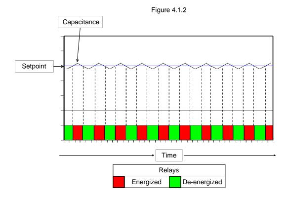
For this reason, a Sensitivity or Hysteresis adjustment has been incorporated in the software. Sensitivity adds a capacitance factor to the baseline. In order for the relays to energize, the sensed capacitance must not only surpass the baseline it must surpass the added capacitance. The set-point plus the sensitivity becomes the switch point. For the relays to de-energize, the sensed capacitance must decrease to less than 1/3 of the sensitivity plus the baseline. (Figure 4.1.3)
