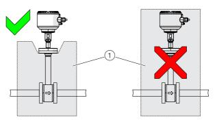
Fig. 8: Insulation of the sensor 1 Insulation
