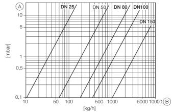
Fig. 9: Pressure loss in logarithmic representation  $\widehat{(A)}$  Pressure loss  $\widehat{(B)}$  Mass flow
