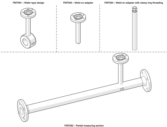
Fig. 2: Pipe components (examples)
