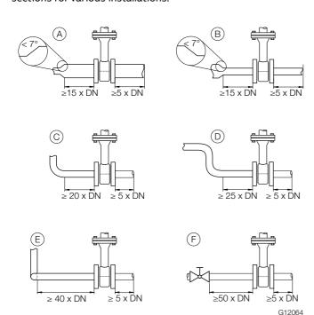
Fig. 6: Inlet and outlet sections
