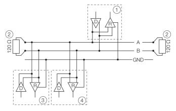
Fig. 25: Communication via the Modbus protocol
