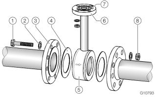
Fig. 13: Installing a pipe component (example, wafer type design)
