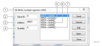
Fig. 29: Write Multiple Registers (example)
