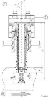
Fig. 17: Integrated changing device in measurement position, dimensions in mm (inch)
