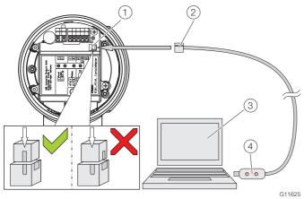
Fig. 30: Connection to the local operating interface
