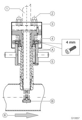
Fig. 35: Gaskets on the changing device
