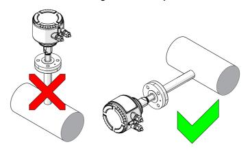
Fig. 7: Mounting position at high ambient temperatures
