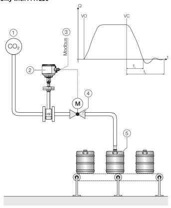
Fig. 32: Filling function FillMass (example  $CO_2$  filling) (1) Gas line ( $CO_2$ ) (2) Sensor (3) Fill start / stop (via Modbus) (4) Fill valve (5) Fill container
