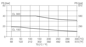
Fig. 11: ASME flange process connection
