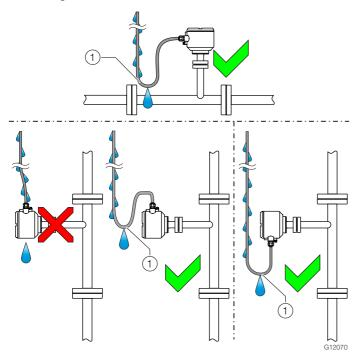
Fig. 22: Laying of the connecting cable 1 Drip loop
