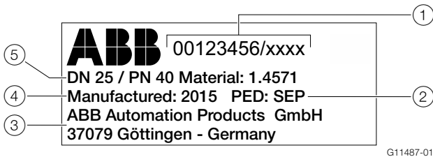
Fig. 5: Factory plate for nominal diameter ≤ DN 25 (example) ① Serial number of the sensor ② Reason for exception under article 4, paragraph 3 of the Pressure Equipment Directive ③ Manufacturer address ④ Year of manufacture ⑤ Nominal diameter / nominal pressure rating and material of the pressure bearing part (wetted part)
