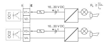
Figure 38: Plug-in card as binary output (I = internal, E = external,  $R_B$  = load)
