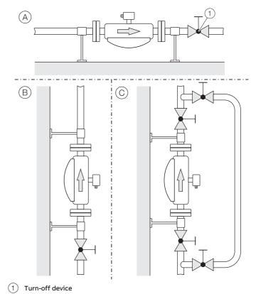
Figure 12: Mounting options for turn-off devices (example)
