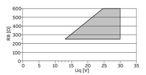
Permissible source voltage  $U_q$  for passive outputs in relation to load resistance  $R_B$  where Imax = 22 mA. Image = -22 Permissible range
