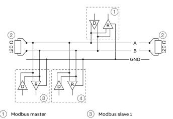
Figure 52: Communication with the Modbus protocol
