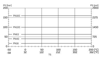
Figure 17: Nickel alloy DIN flange C4 (2.4610) or nickel alloy C22 (2.4602) up to DN 200 (8 in.)
