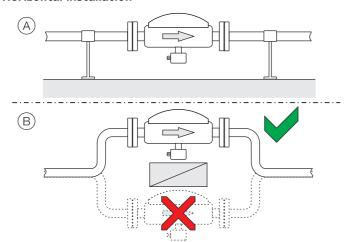
Figure 11: Horizontal installation
