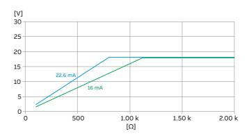
Figure 34: Output voltage dependent on load resistance
