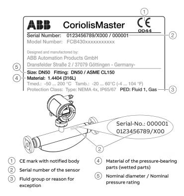
Figure 7: PED marking (example)
