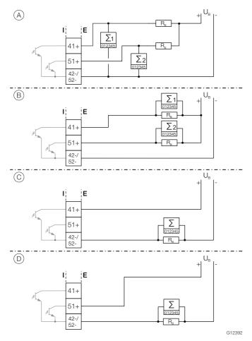
Figure 47: Connection versions digital output 41 / 42 and 51 / 52
