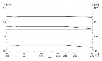
Figure 19: Stainless steel JIS B2220 flange 1.4435 or 1.4404 (AISI 316L) , nickel alloy C4 (2.4610) or nickel alloy C22 (2.4602)
