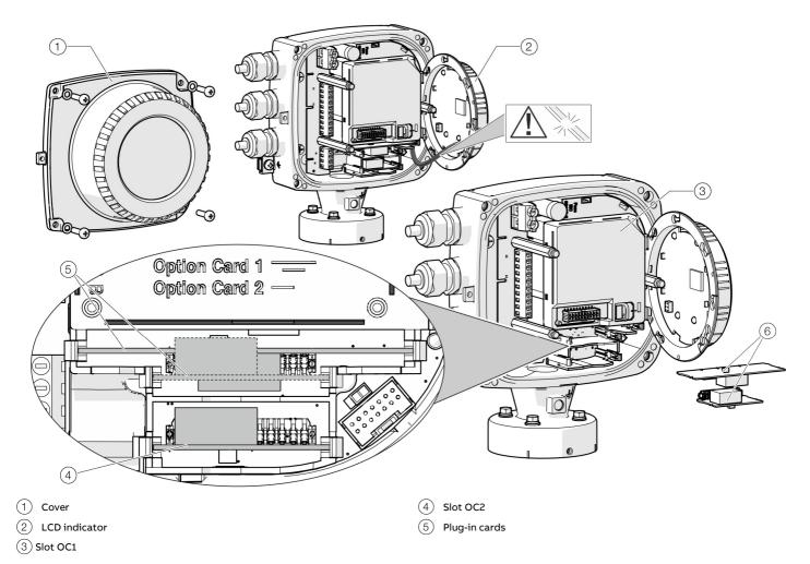
Figure 28: Installation of plug-in cards (example, single-compartment housing)
