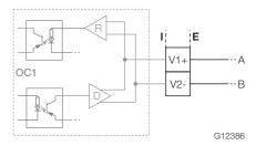
Figure 41: Plug-in card as a Modbus / PROFIBUS DP interface (I = internal, E = external)
