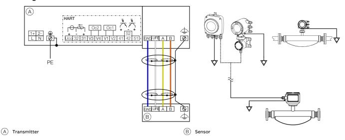
Figure 30: Electrical connection
