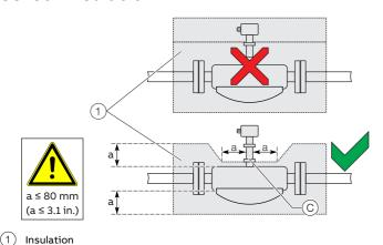
Figure 13: Installation at  $T_{medium}$  –50° to 205 °C (–58 to 400 °F)
