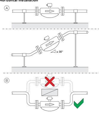
Figure 10: Horizontal installation
