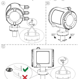
Figure 24: Rotate transmitter housing
