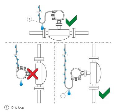
Figure 29: Laying the connection cable
