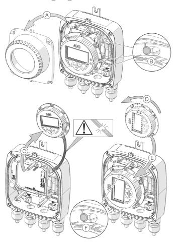
Figure 26: Rotating the LCD indicator
