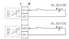
Figure 39: Plug-in card as digital input (I = internal, E = external)
