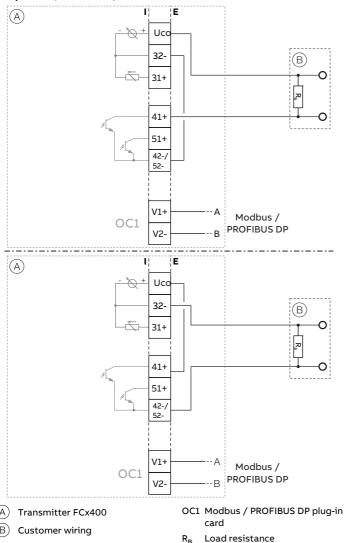
Figure 33: Current output Uco / 32 in power mode
