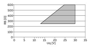
Permissible source voltage  $U_q$  for passive outputs in relation to load resistance  $R_B$  where  $I_{max}$  = 22 mA.  $\blacksquare$  = Permissible range
