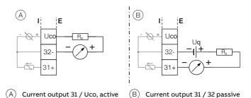
Figure 31: (I = internal, E = external, R<sub>B</sub> = load)
