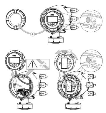
Figure 25: Rotating the LCD indicator
