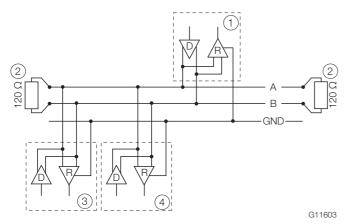
Fig. 23: Communication via the Modbus protocol (1) Modbus master (2) Terminating resistor (3) Modbus slave 1 (4) Modbus slave n ... 32
