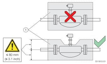
Fig. 13: Installation when  $T_{medium}$  is -50°... 205 °C (-58 ... 400 °F)  $\fbox{(1)}$  Insulation
