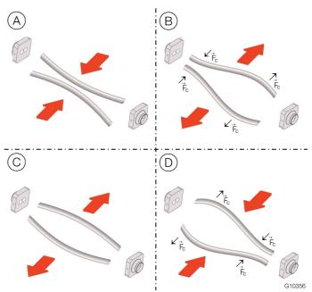
Fig. 3: Simplified representation of Coriolis forces
