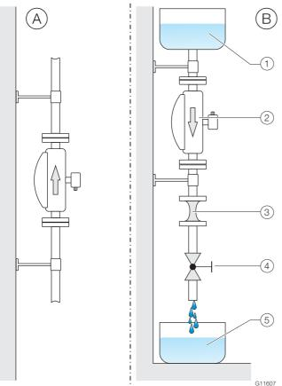
Fig. 8: Vertical installation
