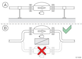
Fig. 10: Horizontal installation
