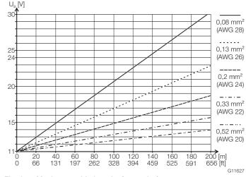
Fig. 25: Maximum cable lengths (examples)  $U_B$  = supply voltage, L = cable length
