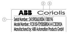
Fig. 27: Modbus address on the name plate (example)
