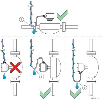
Fig. 20: Laying of the connecting cable (1) Drip loop
