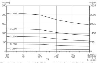
Fig. 16: Stainless steel ASME flange 1.4571 / 1.4404 (316Ti / 316L) up to DN 200 (8")
