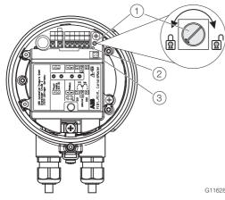
Fig. 26 (1) Write protection switch (2) Service LED
