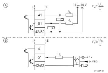
Fig. 22: Passive digital outputs (I = internal, E = external) A Passive digital output 41 / 42 as pulse or frequency output, Passive digital output 51 / 52 as pulse output B Passive digital output 51 / 52 as binary output
