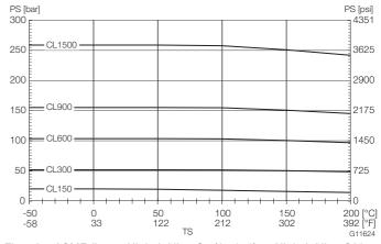
Fig. 18: ASME flange Nickel-Alloy C4 (2.4610) or Nickel-Alloy C22 up to DN 200 (8")
