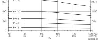
Fig. 15: Stainless steel DIN flange 1.4571 / 1.4404 (316Ti / 316L) up to DN 200 (8")
