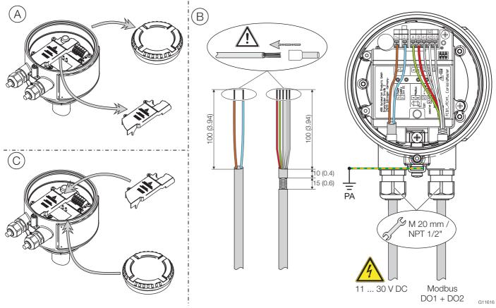
Fig. 24: Connection on the device (example), dimensions in mm (inch) PA = potential equalization
