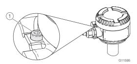
Fig. 19: Cover safety device (example)
