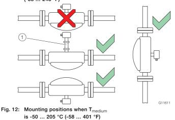
(1) Sensor with option TE1 "extended tower length"
