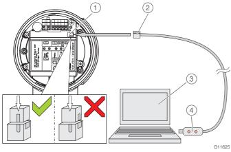
Fig. 29: Connection to the local operating interface
