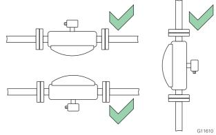
Fig. 11: Mounting positions when T<sub>medium</sub> is -50 ... 120 °C (-58 ... 248 °F)
