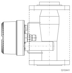
Fig. 14: Insulation of the flowmeter
