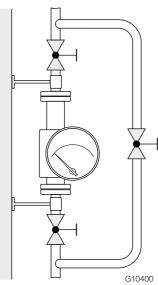
Fig. 13: Installation of the flowmeter (example)
