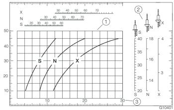
Fig. 17: Flow rate depending on float shape and weight (example)
