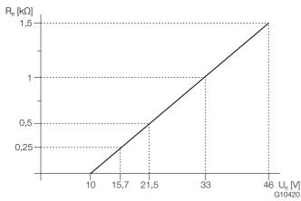
Fig. 25: Load diagram of the current output
