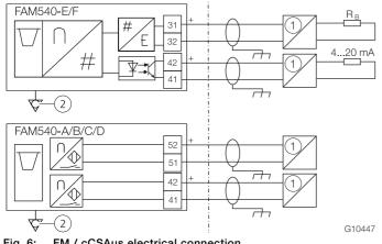
Fig. 6: FM / cCSAus electrical connection (1) FM Approved IS Barrier (2) Potential equalization
