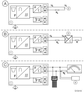
Fig. 24: Analog indicator with transmitter
