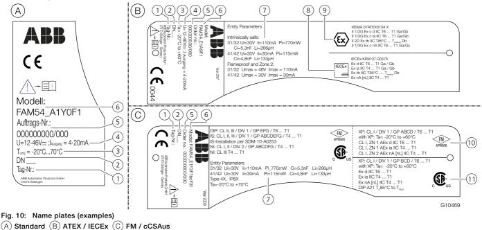
1 TAG number 2 Nominal size and degree of protection 3 Ambient temperature 4 Power supply / output current 5 Order number 6 Model number 7 Electrical data (Ex) 8 IECEx approval 9 ATEX approval 10 FM approval 11 cCSAus approval
