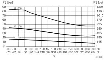
Fig. 20: ASME flange made from stainless steel
