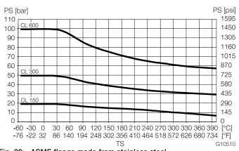
Fig. 22: ASME flange made from stainless steel
