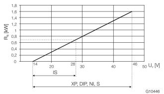
Fig. 7: Terminals 31 / 32, power supply / load  $U_{\rm V}$  Power supply
