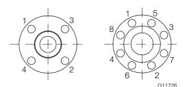
Fig. 18: Tightening sequence for the flange screws
