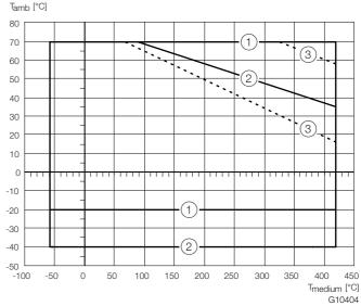
Fig. 15: Medium temperature ( $T_{medium}$ ), ambient temperature ( $T_{amb}$ ) (1) Devices with alarm output -20 ... 70 °C (-4 ... 158 °F)
