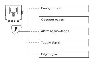
Figure 6 Programmable soft key
