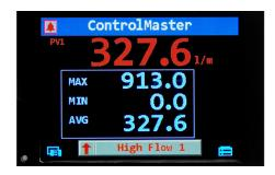
Figure 2 Single PV indication template display
