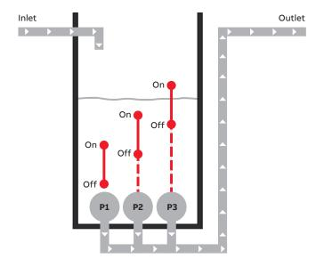
Figure 11 Independent on and off trip points
