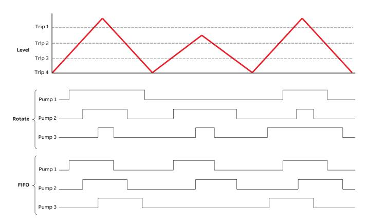
Figure 12 Rotate and FIFO cycling for a 3-pump system
