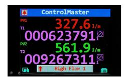
Figure 3 Dual PV and totalization display
