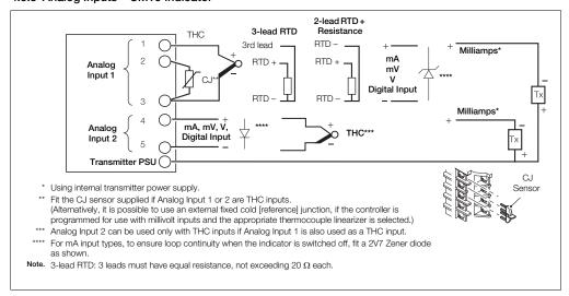
Fig. 4.16 Standard Analog Inputs (1 and 2) - CM15 Indicator
