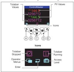
Fig. 3.2 ControlMaster CMF160 Operator Page and Keys
