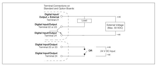
Fig. 4.19 Digital Input and Open Collector Digital Output Connections - CM15 Indicator
