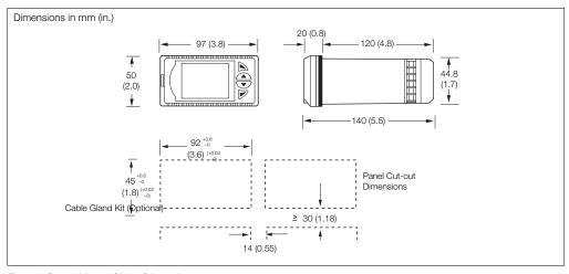
Fig. 4.3 ControlMaster CM15 Dimensions
