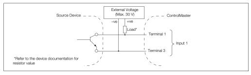
Fig. 4.18 Frequency / Pulse Input - CM15 and CMF160 Indicators
