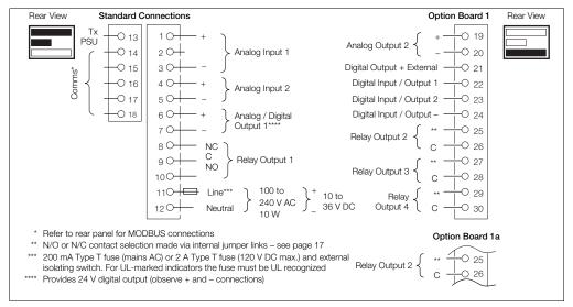
Fig. 4.13 ControlMaster CM15 Electrical Connections
