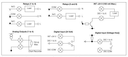
Fig. 4.20 Digital Input / Output, Relays and Analog Output Connections - CMF160 Indicator
