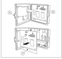
Fig. 4.12 Accessing the CMF160 Indicator Connection Board
