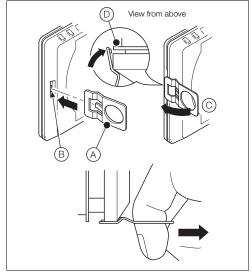
Fig. 4.10 Removing the CM15 Indicator from the Case
