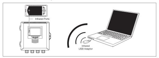
Fig. 9.1 PC Configuration via Infrared Port
