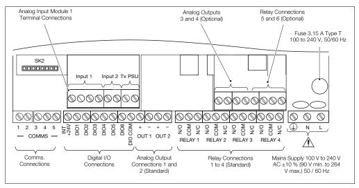
Fig. 4.15 ControlMaster CMF160 Terminal Connections
