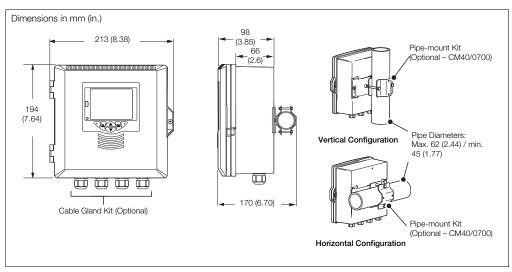
Fig. 4.5 ControlMaster CMF160 Pipe-mount Option
