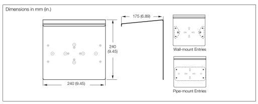
Fig. 4.7 ControlMaster CMF160 Weathershield (CM40/0702) - Pipe- and Wall-mount (CM40/0700) Options
