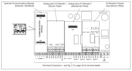
Fig. 4.14 ControlMaster CMF160 Module Locations
