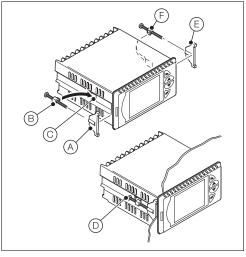
Fig. 4.8 Mounting Details - CM15 Indicator
