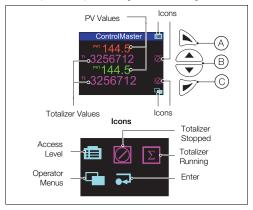
Fig. 3.1 ControlMaster CM15 Operator Page and Keys
