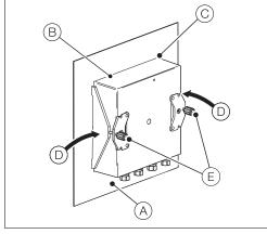
Fig. 4.9 Mounting Details - CMF160 Indicator
