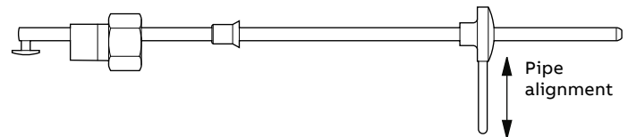
Figure 15 Pipe-bore gauging tool
