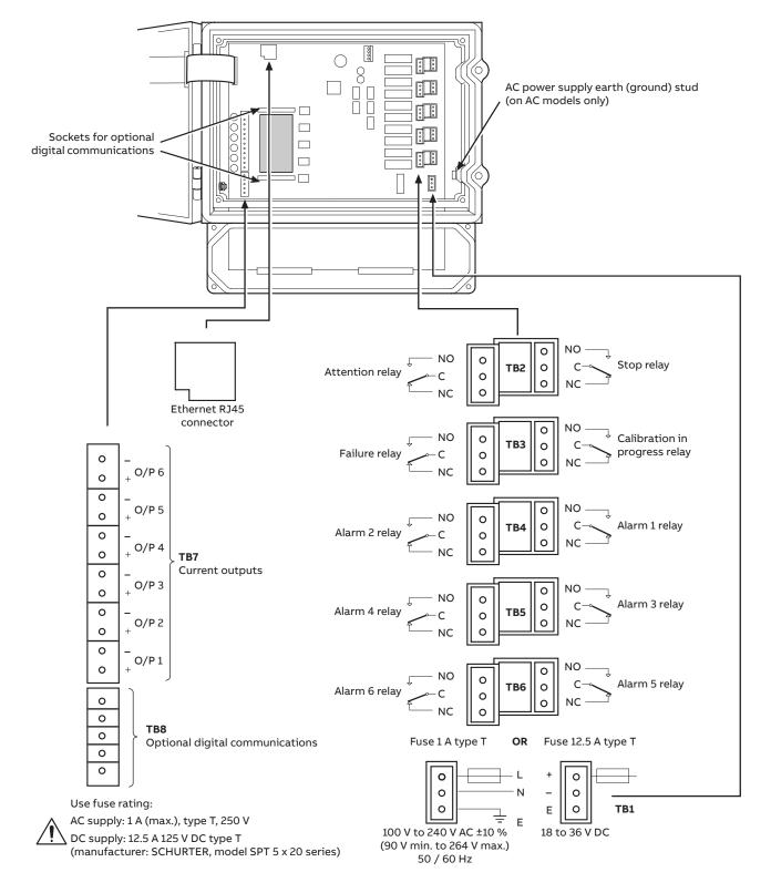
Fig. 6 Electrical connections
