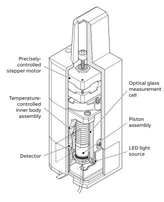
Fig. 1 Measuring head detail
