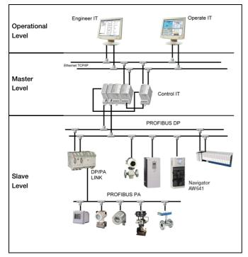
Fig. 2.1 Typical Profibus Network
