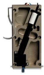
Figure 3 Electrode in temperature-controlled flow cell
