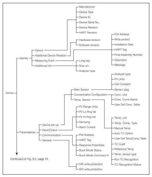
Fig. 9.1 ACA592 2-Electrode Conductivity Transmitter - HART Configuration Parameters
