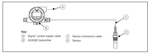
Fig. 3.2 Installation in Non-Hazardous Area
