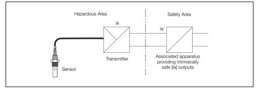
Fig. 4.9 Intrinsic Safety - ATEX/IEC Ex
