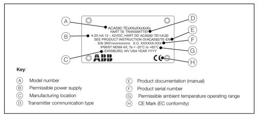
Fig. 3.6 Example of ACA592 2-Electrode Conductivity Transmitter Label
