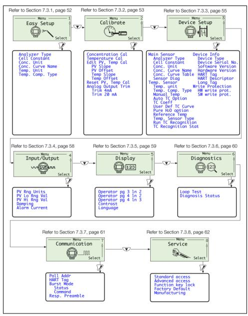
Fig. 7.4 ACA592 2-Electrode Conductivity Transmitter - Concentration Parameter Map
