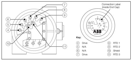
Fig. 4.3 ACA592-TE 2-Electrode Conductivity Transmitter - Sensor Connections at Transmitter Terminals
