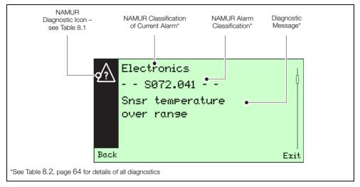
Fig. 8.1 Example of Diagnostic Alert
