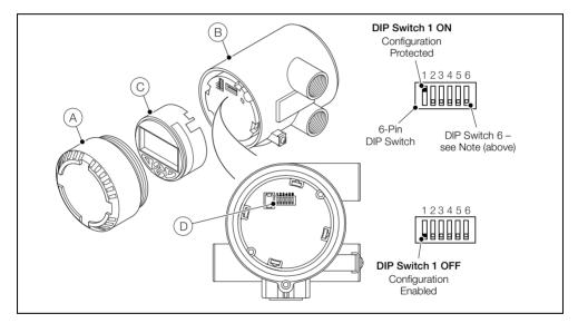
Fig. 6.2 Configuration DIP Switch
