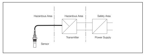
Fig. 4.11 Type n (Non-sparking) – ATEX/IEC Ex
