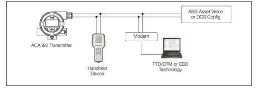
Fig. 6.1 Configuration Options - Schematic
