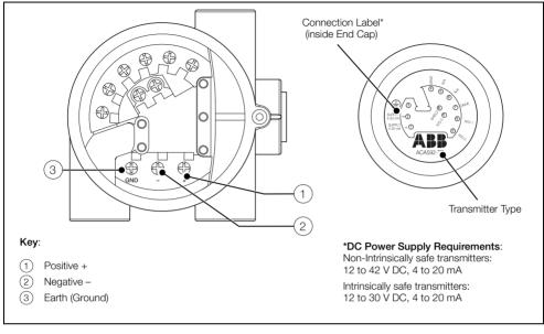
Fig. 4.2 Power Supply Connections at Transmitter Terminals
