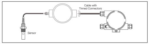
Fig. 4.5 Sensor with Junction Box and Extension Cable
