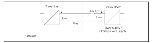
Fig. 4.7 Standard Application with HART Functionality
