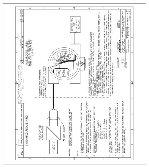
Fig. B.3 Installation Drawing P0910
