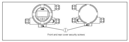
Fig. 3.1 Transmitter Cover Security Screws
