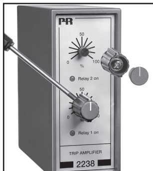
Picture 2: Removal of knobs.
